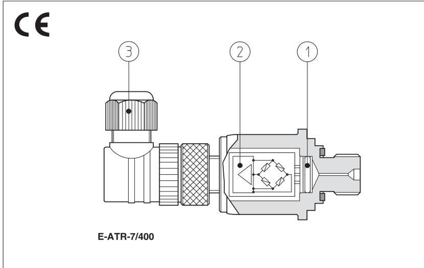
E-ATR-7 pressure transducers measure the static and dynamic pressure of the hydraulic fluid, supplying a voltage or current output signal.
