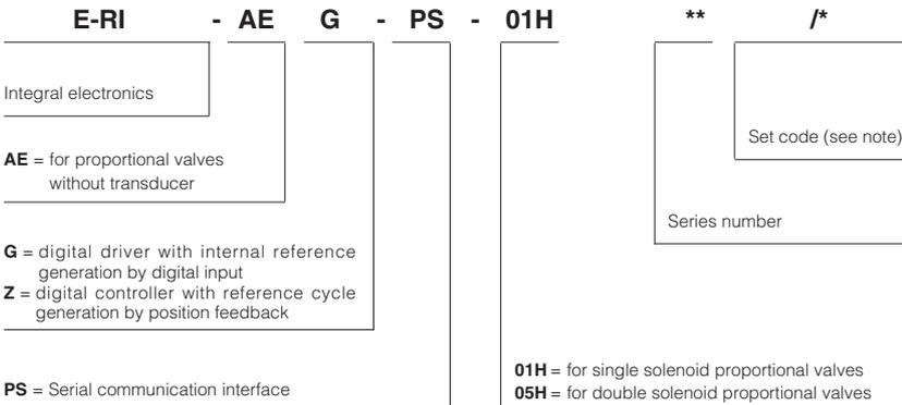
**Note:** the set code identifies the correspondance between the digital integral driver and the relevant valve; it is assigned by Atos when the driver is ordered as a spare part.
