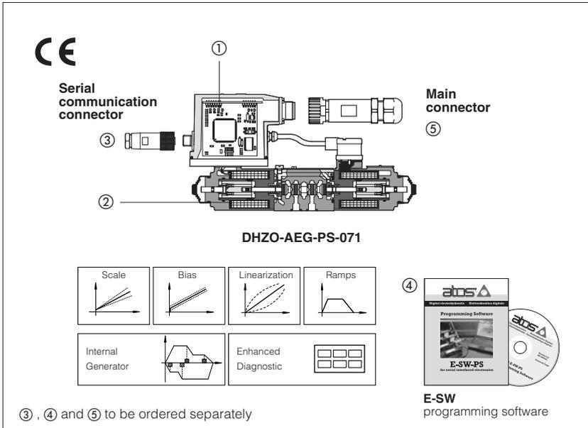
The driver ① supplies and controls the current to the solenoid of Atos proportional directional valves without transducer according to the internal reference signal.
