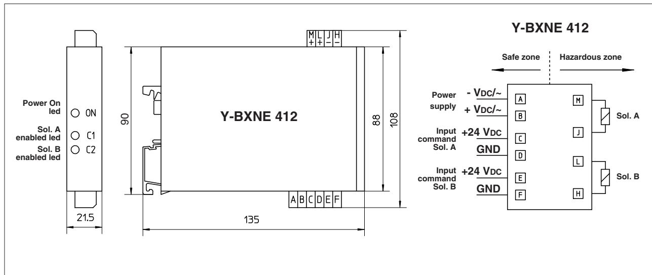
**22** EXTERNAL PROFILE OF INTRINSICALLY SAFE VALVES [mm]
