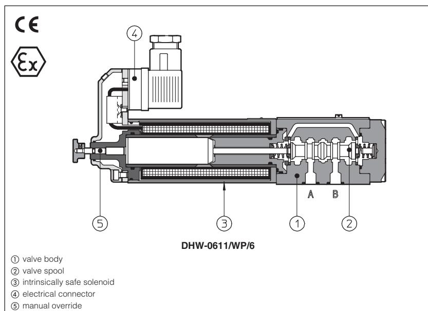
On/off valves equipped with intrinsically safe solenoids certified according to ATEX 94/9/CE, protection mode:
