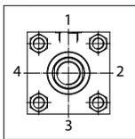
FRONT HEAD: **B1** = oil port position; **E\*** = cushioning adjustment position
