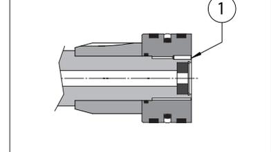
L<sub>f</sub> is the total cushioning length. When the stroke-end cushionings are used as safety devices, to mechanically preserve the cylinder and the system, it is advisable to select the cylinder's stroke longer than the operating one by an amount equal to the cushioning length L<sub>f</sub>; in this way the cushioning effect does not influence the movement during the operating stroke.
