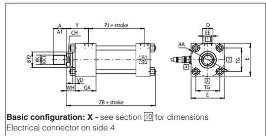
**12 MOUNTING STYLES FOR SERVOCYLINDERS TYPE CKN**
